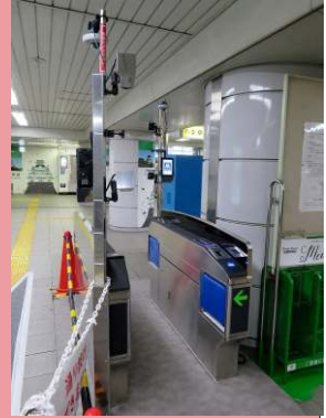
Automatic ticket gate with face recognition system in Osaka Metro Morinomiya
